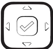
**Navigation/Select Keys** - Pressing the UP and DOWN keys lets you view different status and text messages on the LCD display (if there is more than 1 line of status/text messages). These buttons also let you scroll through menu selections, such as the Options List.
