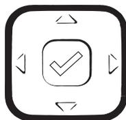
**Navigation/Select Keys** - Pressing the UP and DOWN keys lets you view different status and text messages on the LCD display (if there is more than 1 line of status/text messages). These buttons also let you scroll through menu selections, such as the Options List.
